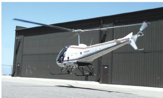
Figure 2. Exercise extreme caution when hovering near buildings or other aircraft.
